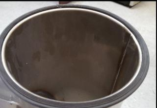
A flexible V-shaped gasket fits over the Vanstone edge on one end of the pipe. Only one gasket per joint is required.
